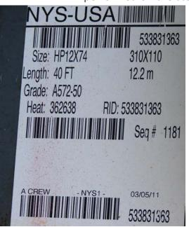
b) Materials descriptions, quantities, and means of material identification such as heat numbers, lot numbers, and other industry identification markings for each process the material underwent so the final product can be tracked through a step process from smelting to final product.
